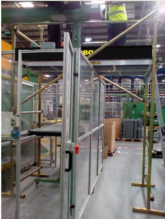
The LOBO System is a versatile work platform product that combines the flexibility and strength of traditional scaffolding with the simplicity and mobility of tower systems.
