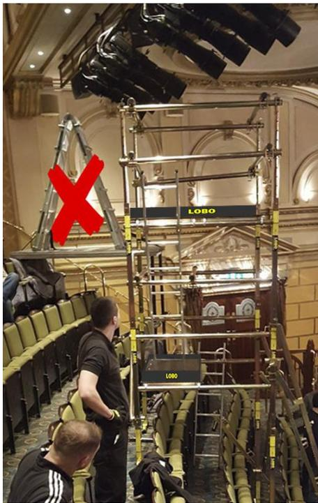
The unique and patented hand adjustable clamp, when combined with the tube, allows the technician or engineer to create a work platform, of any shape or size, without the need for any tools.
