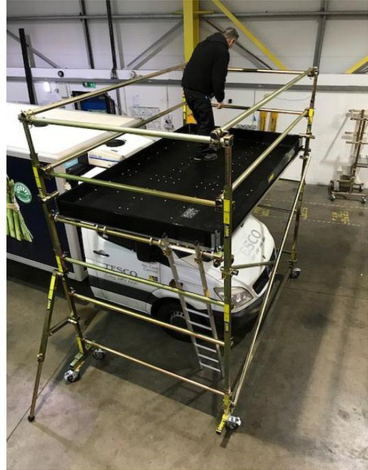
The LOBO System can be transported from site and assembled with ease from a flat pack, into any required configuration, by your own service engineers. Or it can be stored in a LOBO Towerstore unit when not in use.
