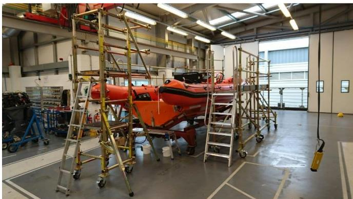
b) The LOBO System is a rigid and stable product, which meets or exceeds current safety regulations. Handrails can be fitted in seconds, at any point in the erection process.
