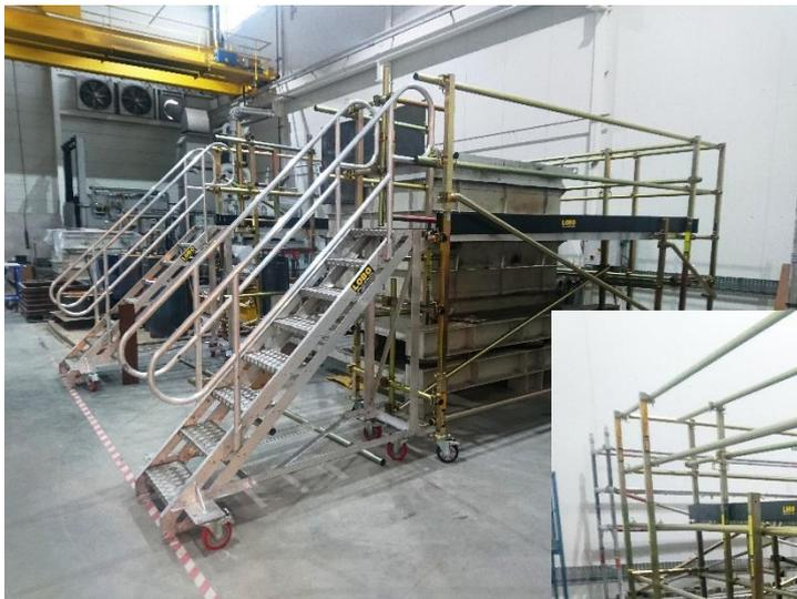
The system is made from modular steel components, which are easy and quick to assemble. It flat packs for transportation and yet is incredibly strong.
