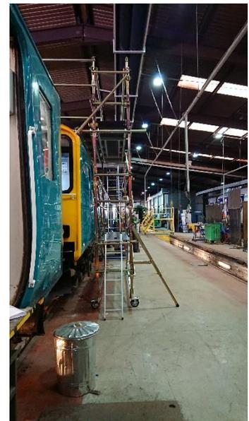
Maintenance crews can attach a handrail around the carriage or at any point across the roof, from a lower level. This ensures a safe system is assembled while personnel are not exposed to the risk of a fall during assembly while using the system for maintenance.
